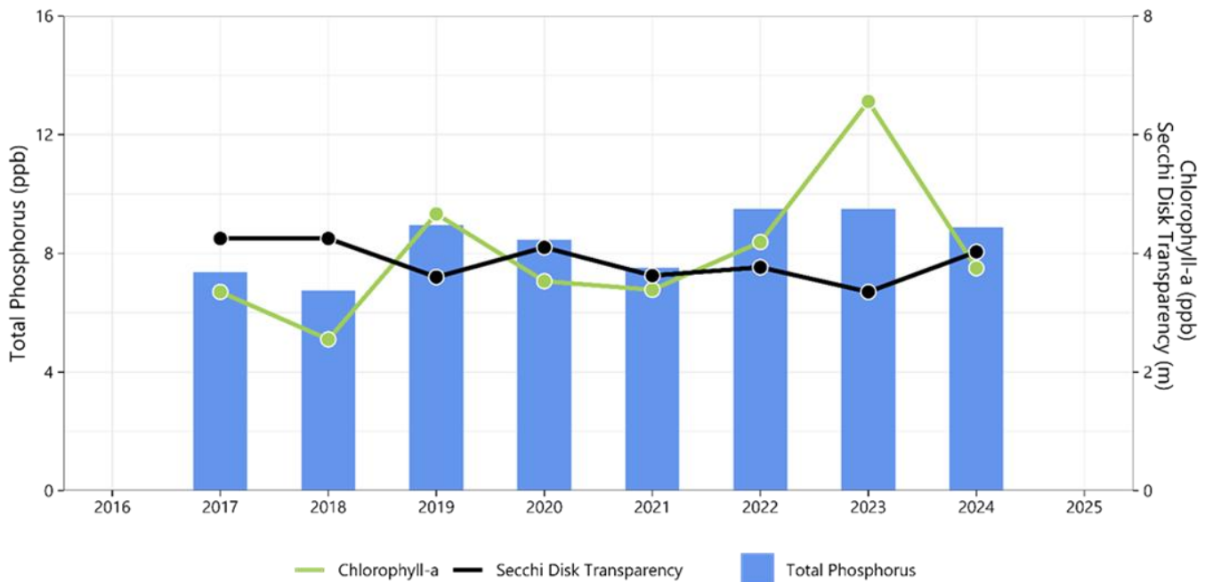
Figure 5. Median surface (0-3 meters) or composite total phosphorus (n=28), median composite surface (0-3 meters) chlorophyll-a (n=32), and median water clarity (Secchi Disk depth, methods not recorded) (n=25) measured at the deep spot of Shaws Pond [1 DEEP] largely in June-September from 2017 to 2024. No statistically significant trends were detected from the Mann-Kendall nonparametric trend test using rkt package in R Studio, though 10 or more years of data are preferred to confidently detect trends.
